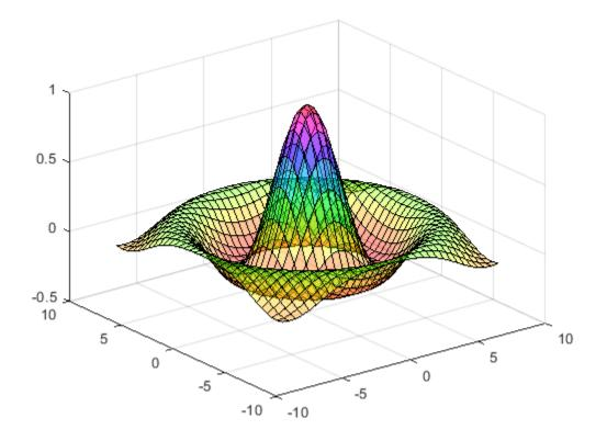
MATLAB displays a surface with a face alpha value of 0.4. Alpha values range from 0 (completely transparent) to 1 (not transparent).
