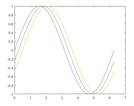
The legend function provides an easy way to identify the individual lines: legend( $'\sin(x)', '\sin(x-.25)', '\sin(x-.5)'$ )
