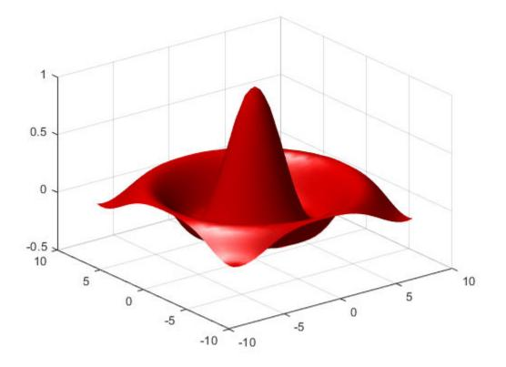
Lighting is the technique of illuminating an object with a directional light source. In certain cases, this technique can make subtle differences in surface shape easier to see. Lighting can also be used to add realism to three-dimensional graphs.
