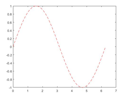
'r--' is a *line specification*. Each specification can include characters for the line color, style, and marker. A marker is a symbol that appears at each plotted data point, such as a +, o, or \*. For example, 'g:\*' requests a dotted green line with \* markers.
