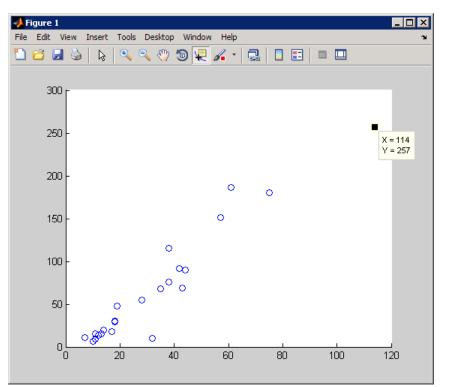
Select the Data Cursor Tool  $\blacksquare$  and click the rightmost data point. A datatip displaying the point's x and y value is placed there.
