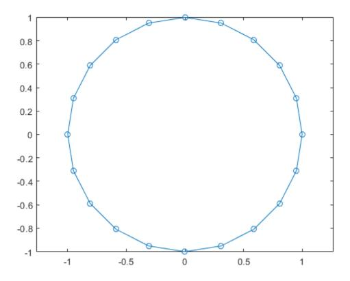
The axis equal command makes the individual tick-mark increments on the *x*- and *y*-axes the same length, which makes this plot more circular in appearance.
